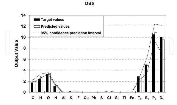
Fig. 13. Examples of rocket motor parameter predictions DB-class rockets obtained for the overall optimum NNPLS model trained with 3 latent dimensions on all data points.
