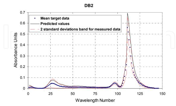
Fig. 7. Examples of plume irradiance predictions for 'unseen' DB-class rocket motors obtained during leave-one-out cross-validation of NNPLS with 11 latent dimensions.
