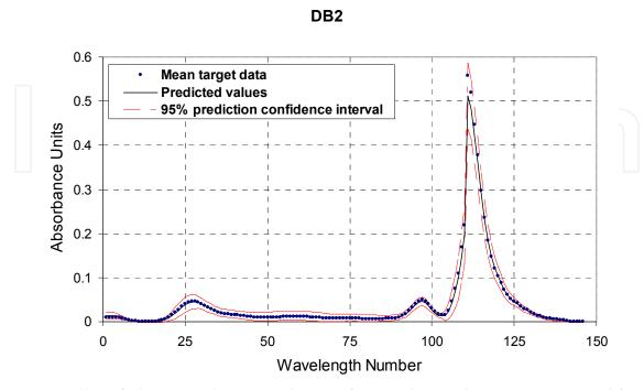
Fig. 9. Examples of plume irradiance predictions for DB-class rocket motors obtained for the overall NNPLS model using 11 latent dimensions.
