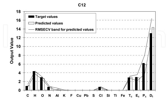
Fig. 12. Examples of rocket motor parameter predictions for 'unseen' rocket motors in the C-class obtained during leave-one-out cross-validation of the NNPLS model (3 latent dimensions).
