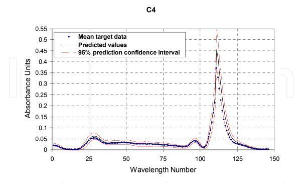
Fig. 10. Examples of plume irradiance predictions for C-class rocket motors obtained for the overall NNPLS model using 11 latent dimensions.
