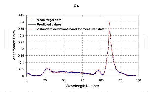
Fig. 8. Examples of plume irradiance predictions for 'unseen' C-class rocket motors obtained during leave-one-out cross-validation of NNPLS with 11 latent dimensions.
