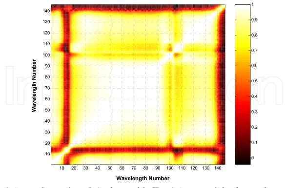
Fig. 3. A map of squared correlation factors of the IR emission spectral absorbance values to investigate the presence of potentially redundant correlated information in the variable space.
