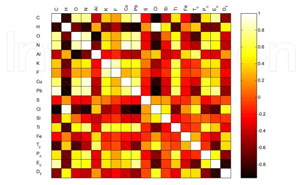
Fig. 4. A map of correlation factors of the rocket motor design parameters and chemistry to investigate the presence of potentially redundant correlated information in the underlying structure.
