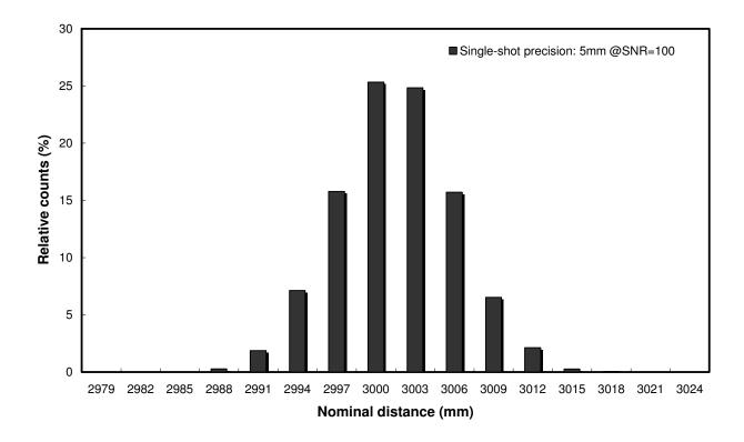
Fig. 11. Distribution of single-shot measurements for a target placed at a nominal distance of 3m from the instrument. SNR: 100. Frequency of acquisition: 400 kHz
