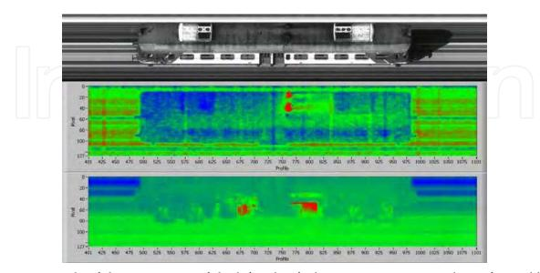
Fig. 5. Example of the acquisition of the left side of a locomotive concurrently performed by the upper image acquisition system, and the upper and lower thermal monitoring systems.
