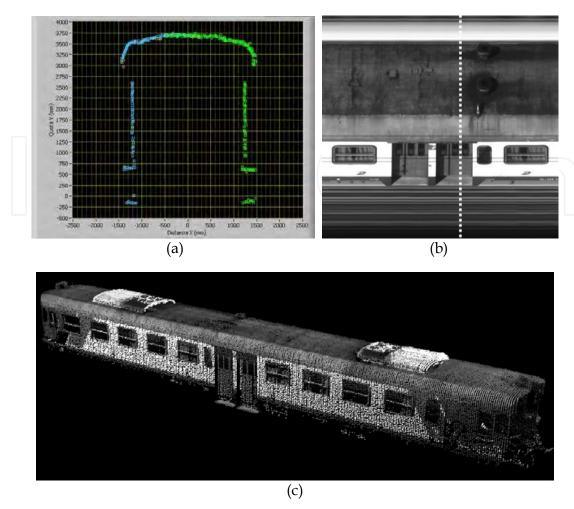
Fig. 13. (a) Acquisition of a single profile of the locomotive shown in Fig. 5; (b) detail of the visual image of the locomotive, highlighting the acquired profile; (c) 3D profile the entire locomotive as obtained by the elaboration of the telemeter measurements.
