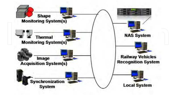
Fig. 2. Overall architecture of a Railway Multifunction Portal
