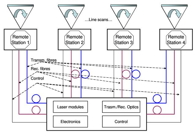
Fig. 7. Overall layout of the telemeter.
