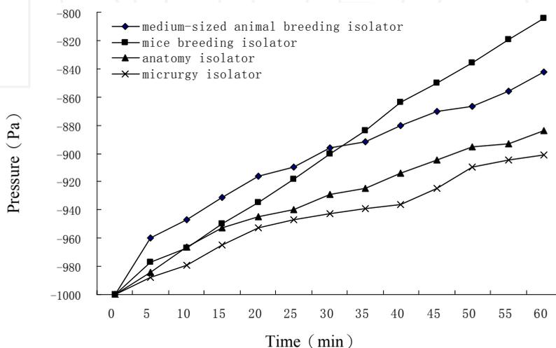
Fig. 2. Negative 1000Pa pressure decay test of isolator.
