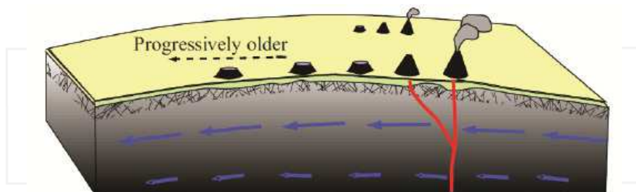
Fig. 2. The hotspot concept: the hotspot tracks are due to the drifting of a plate over a stationary mantle source. The plate displacement pushes the old volcanoes away from the source as young volcanoes are formed above the source- from Clouard (2001)
