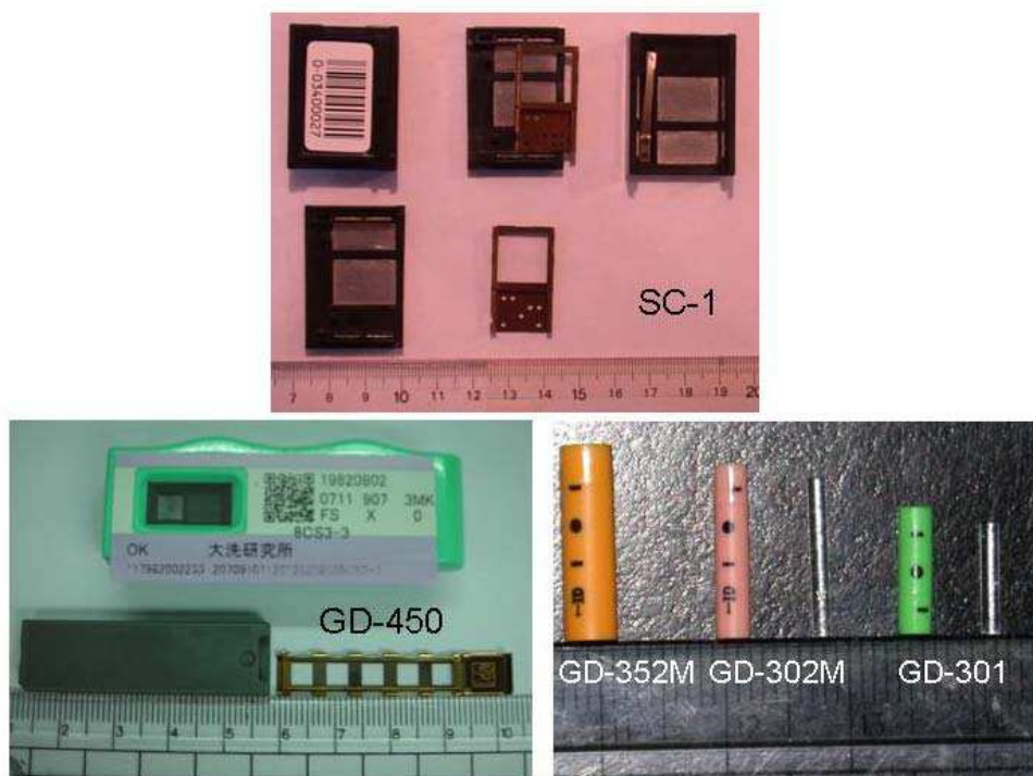
Fig. 7. Three types of RPLGD; above: SC-1 system for environmental radiation monitor; below left: GD-450 system for personal dose monitor; and below right: small volume Dose Ace system for research
