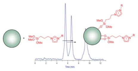
Fig. 12. Chromatogram of amixture of acids eluted using 5 mM phosphate at pH 4.2 in an MPIM-modified silica particle packed column, using UV detection at a wavelength of 214nm. Flow rate is 200 mL/ min. Peaks, from left to right: 3-(p-hydroxyphenyl) propionic acid (10mM), p-hydroxyphenylacetic acid (10mM), and benzoic acid (10mM) (Wang et al., 2006).
