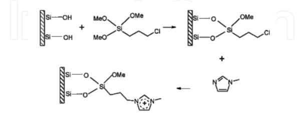
Fig. 13. Scheme representation of the IL coating procedure (Qin & Li, 2002).
