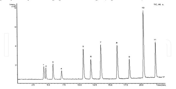
Fig. 9. Gradient separation of the test mixture. Column RP C<sub>8</sub> MetaSil Basic 250×4.6 mm I.D. 5  $\mu$ m (Varian). Mobile phase A, acetonitrile; B, water (1% acetic acid/20 m M ammonium acetate) 0 min. 10% B, 10 min. 20% B, 25 min. 50% B.1-EEIM Br, 2- PMIM Br, 3- PEIM Br, 4- BMIM Cl, 5- BZMIM BF<sub>4</sub>, 6-AMIM Cl, 7- EBZMIM Cl, 8- pMBZMIM Cl, 9-HMIM Cl, 10- HEIM Cl, 11- HpMIM Cl. (Stepnowski et al., 2003).
