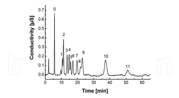
Fig. 8. Chromatogram of separation of ionic liquid cations mixture with isocratic elution for mobile phase consisting of 30% v/v of acetonitrile and: 70% v/v of 5mM MSA (methanesulfonic acid). Key:0–unknown compound,1–EEIM,2–PMIM,3–BMIM,4–BEIM,5–MBPy,6 – AMIM, 7 – BzMIM, 8 – EBzMIM, 9 – HMPy, 10 – HMIM, 11 – OMIM. The cations of IL were analyzed on a Dionex IonPac CS15 column (250mm x 8.5mm) (Molikowa et al., 2010).
