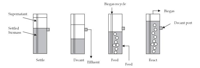
Fig. 6. Anaerobic sequencing batch reactor (adapted from Khanal, 2008)
