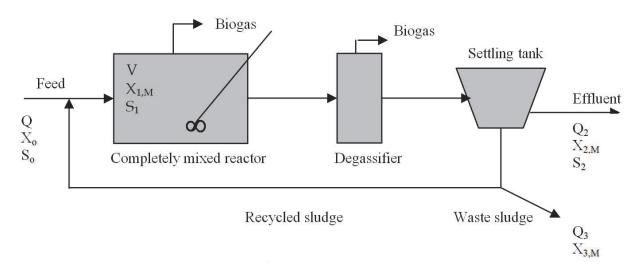
Fig. 7. Anaerobic contact process (after Khanal, 2008)
