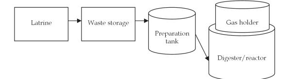
Fig. 3. Schematic of a small-scale biogas production system (adapted from NAS, 1977)
