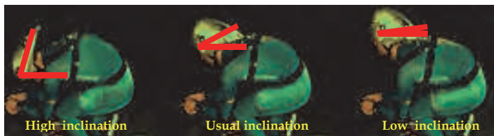
Fig. 11. Inclination of the head in time trial and corresponding inclination of the helmet (Wind tunnel of Marseille, France).
