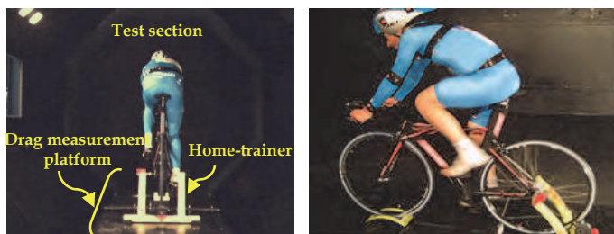
Fig. 17. Measuring device for the assessment of the drag applied on a time trial cyclist.
