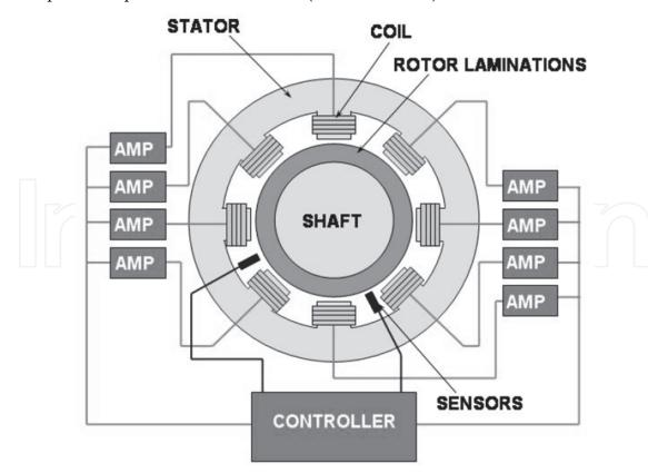
Fig. 7. Schematic of an Active Magnetic Bearing (Clark et al., 2004).
