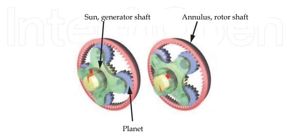
Fig. 2. Planetary gearing system.
