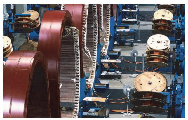
Fig. 4. Multipole annular generators under assembly (Photo: Enercon).
