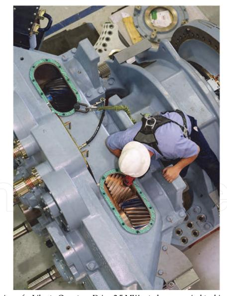
Fig. 1. Top view of a Liberty Quantum Drive 2.5 MW rated power wind turbine gearbox (Source: Clipper Windpower).
