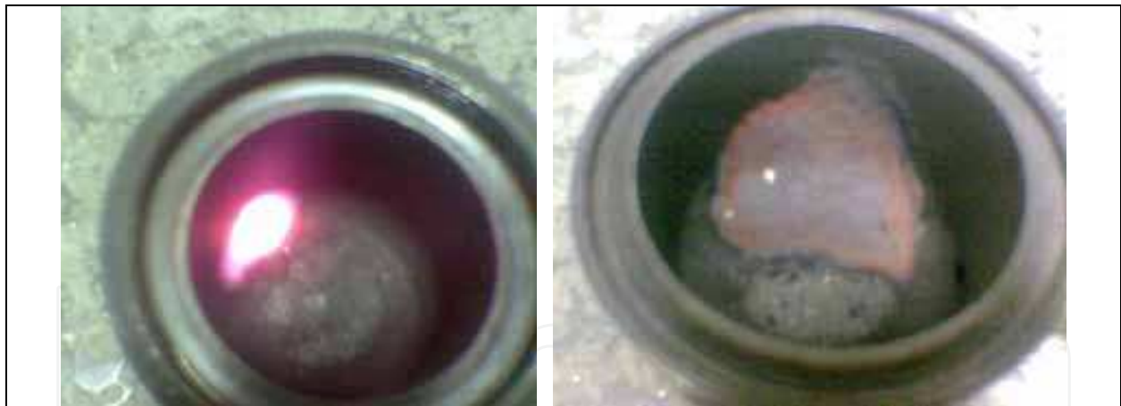
Fig. 14. Images of opened vial during combustion reaction of 3Fe 2 O 3 +8Al powder mixture.
