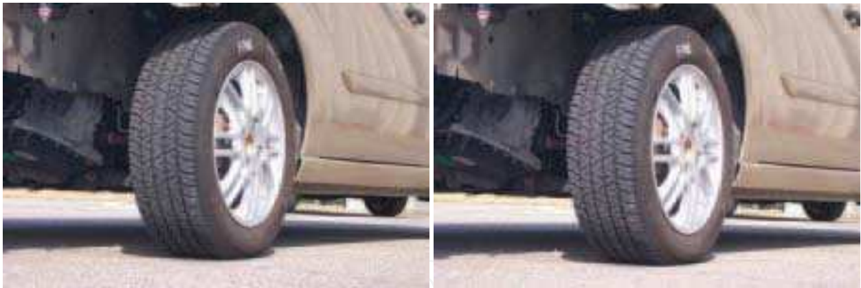
Fig. 1. A fully inflated tire (left) and one with only 70% pressure (right) (David, 2004)
