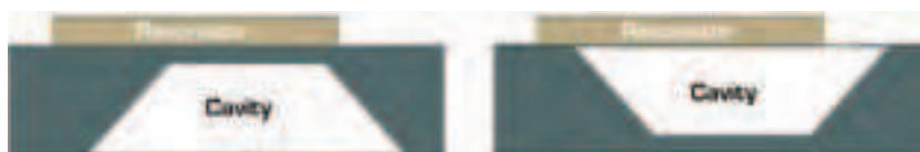
Fig. 14. FBAR processes: (a) Substrate etching (b) Substrate micro-machining.
