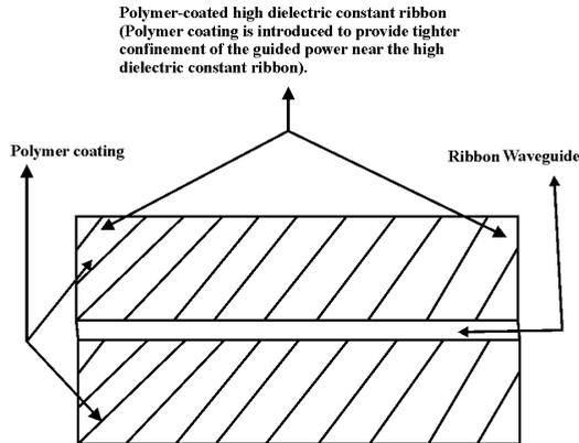
Fig. 20. (a): Longitudinal cross-sectional geometry of a polymer-coated high dielectric constant ribbon. The thickness and width of the high dielectric constant ribbon are, respectively,  $0.0635\lambda_0$ . The dielectric constant of the ribbon is 10 while that of the polymer is 2.04 [35].
