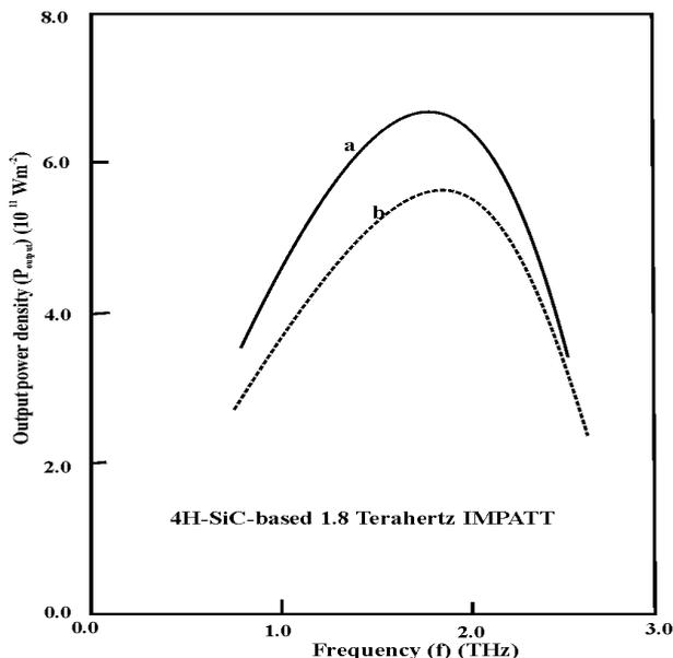
Fig. 9. (b): Effect of series resistance on output power density ( $P_{max}$ ) of SiC THz IMPATT diodes. (a) 4H-SiC IMPATT at 300K,  $R_s=0.0\Omega$ , (b) 4H-SiC IMPATT at 300K,  $R_{s,total}=2.2 \times 10^{-11} \Omega \text{ m}^2$
