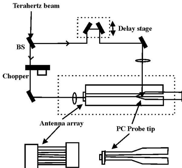
Fig. 21. Detection of Terahertz beam by photo-conductive method
