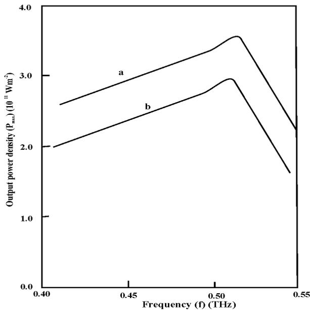
Fig. 9. (a): Effect of series resistance on output power density  $P_{max}$  of 4H-SiC 0.5 THz IMPATT diode. (a) 4H-SiC IMPATT at 300K,  $R_s=0.0\Omega$ , (b) 4H-SiC IMPATT at 300K,  $R_{s,total}=0.386 \times 10^{-9} \Omega \text{ m}^2$
