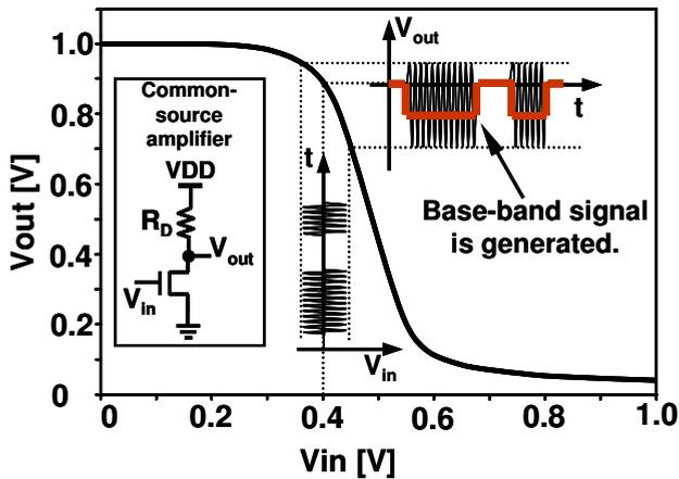
Fig. 33. Nonlinear pulse detection using a common-source amplifier.
