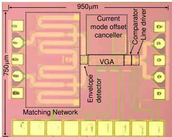
Fig. 43. Chip micrograph.
