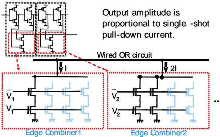
Fig. 5. MOSFET sizing for generating pseudo-raised cosine pulse.
