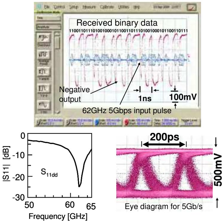
Fig. 44. Summary of measured results of the receiver.
