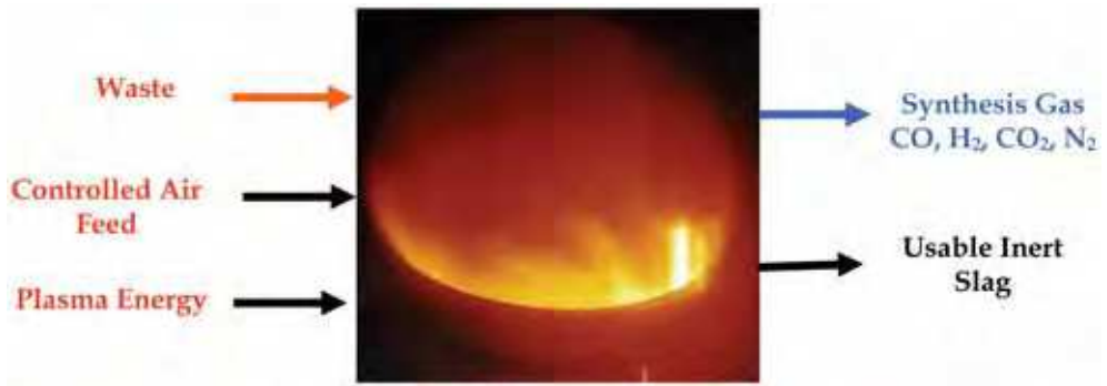
Fig. 10. A schematic diagram of plasma process
