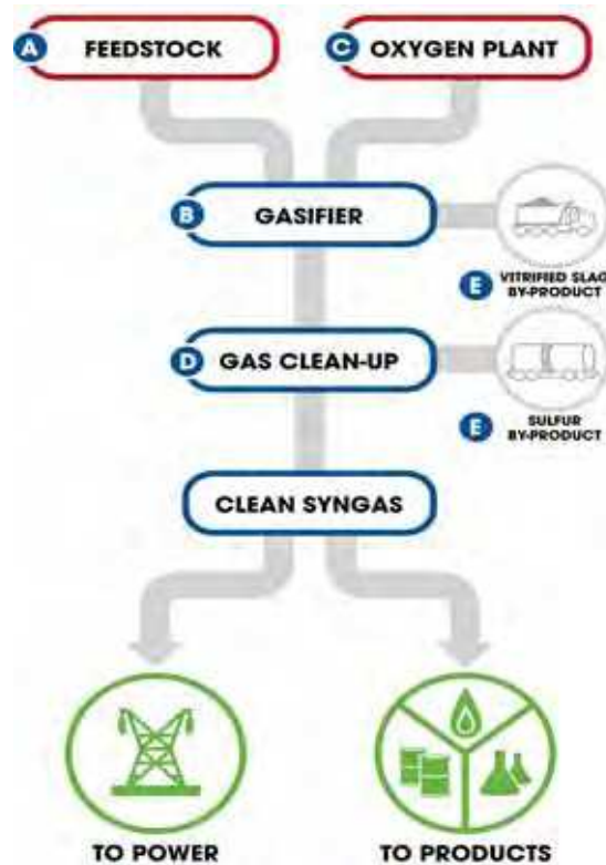
Fig. 7. A schematic diagram of gasification process
