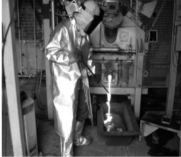
Photo 11. Tapping inert slag (Pyrogenesis Canada Inc, Montreal, Canada)
