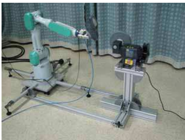
Fig. 5. Experimental cell for shoe bottom roughing
