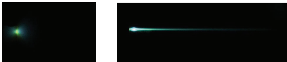
Fig. 7. Plasma images without (left) and with (right) horizontal magnetic field
