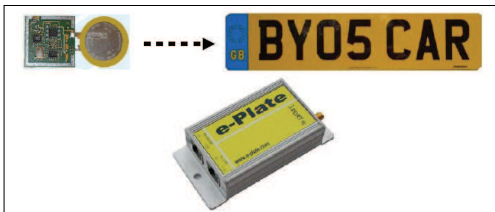
Fig. 3. RFID tag by Hill Numberplates Ltd and e-Plate reader by i-Port
