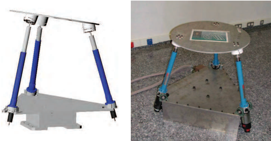
Fig. 1. The 3-DOF RPS parallel robot; ADAMS model on the left and Actual 3-RPS parallel robot on the right (built at the Polytechnic University of Valencia).
