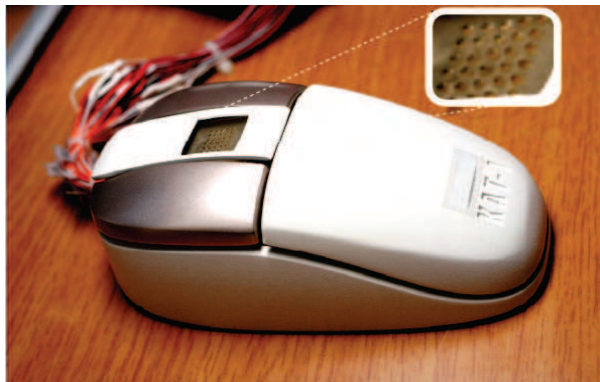
Fig. 3. A prototype of the texture display mouse
