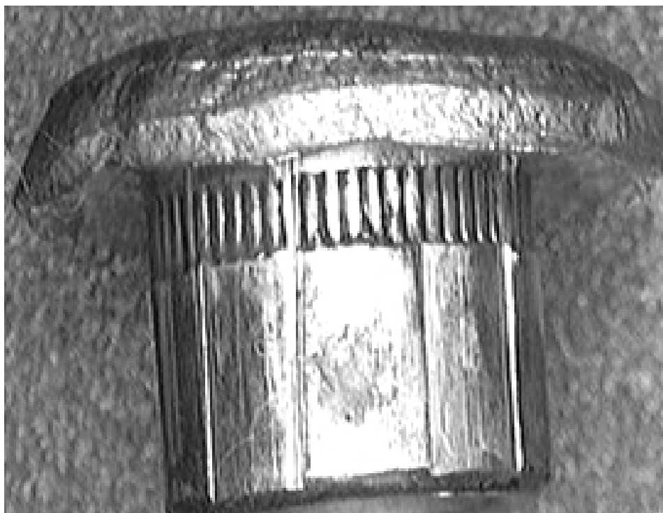
Fig. 1. Landmarks and groove marks of a fired projectile
