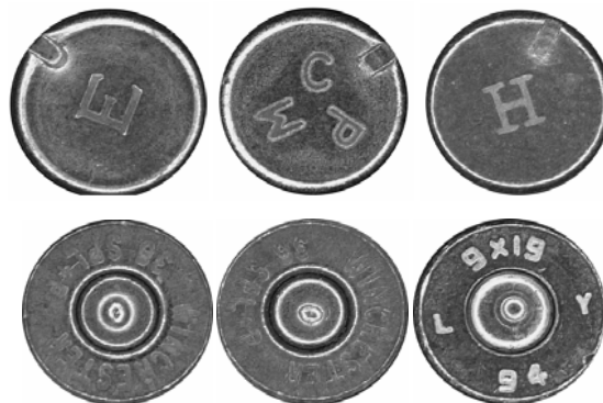
Fig. 14. Rim-firing, first row; Center-firing, second row.
