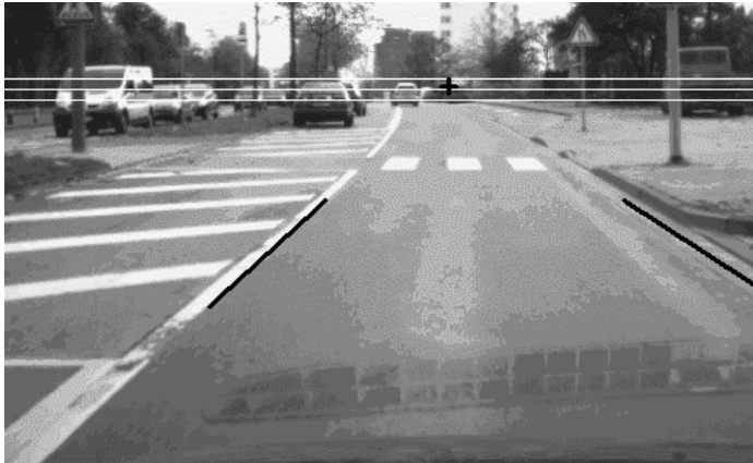
Fig. 6. Linear lane detection result
