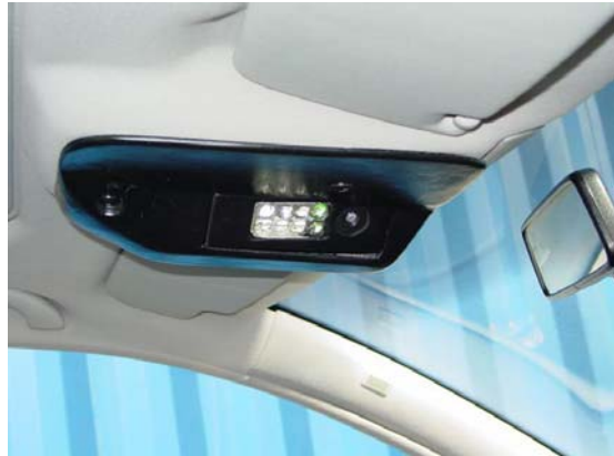
Fig. 4. Smart airbag application using a PMD TOF vision systems (Husmann & Hess, 2006)
