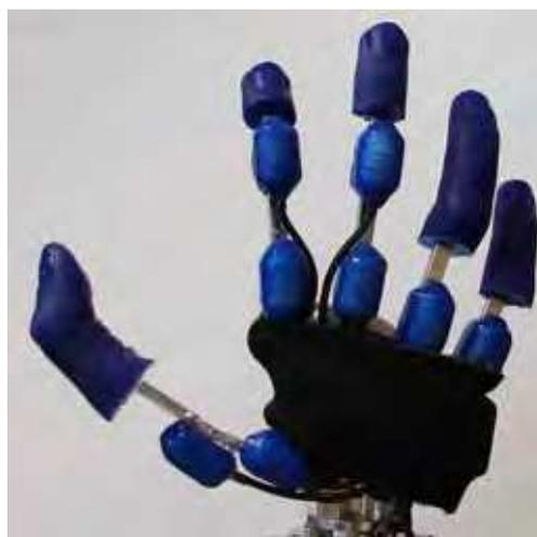
Fig. 3. Current prototype of a fluid hand
