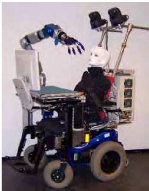
Fig. 10. Rehabilitation Robot FRIEND-II with fluidic Hand.
