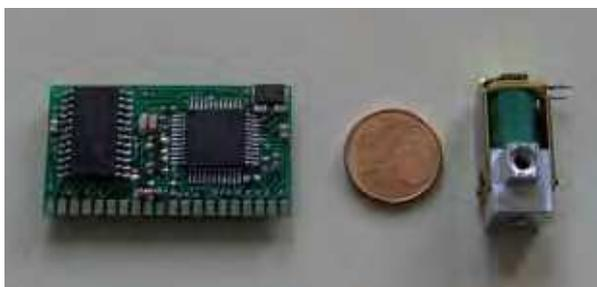
Fig. 4. Electric valve and control unit.
