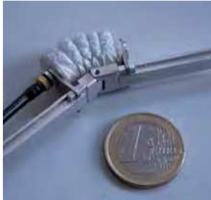
Fig. 2. Flexible fluidic actuator with artificial joint.
