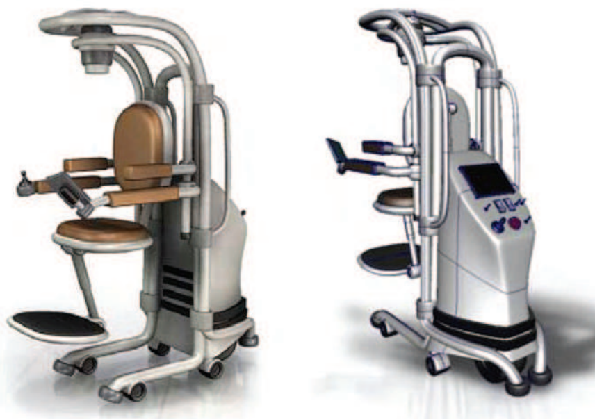
Fig. 15. Front (left) and rear (right) concept drawings of the HLPR Chair as a more ergonomic and commercialized version.
