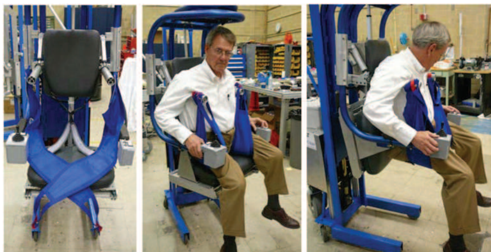
Fig. 14. Photographs of the HLPR Chair sling showing (left) the sling ready for the patient to be seated, (center) a patient with the sling ready to lift while seated on the HLPR Chair seat, and (right) the patient fully supported by the sling with the HLPR Chair seat rotated behind the patient.
