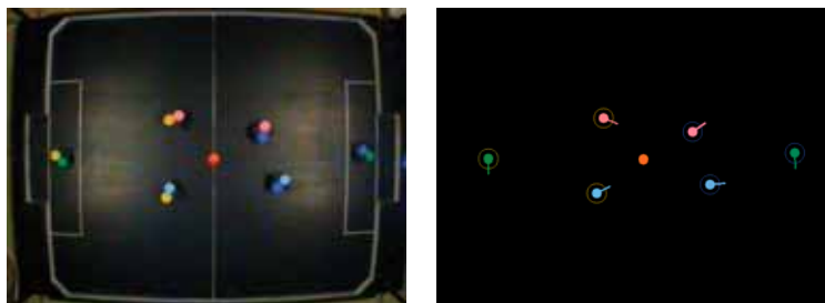
Fig. 10. (left) Captured image containing a ball and two complete teams of robots and (right) result of the execution of the system, showing the computed position of each object
