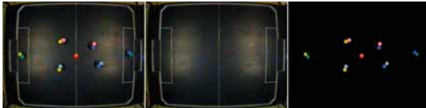
Fig. 5. (left) Captured image containing a ball and two complete teams of robots (center) background and (right) result of background subtraction
