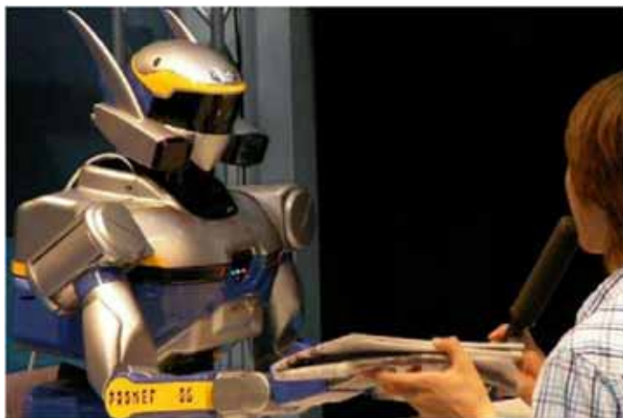
Fig. 1. Humanoid robot HRP-2 interacting with a user using vision and speech information
