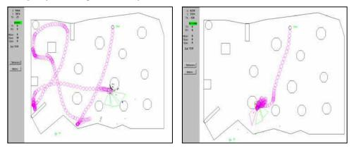
Fig. 9. Trajectories of the robot obtained by FQL algorithm using a random initialization of parameters
