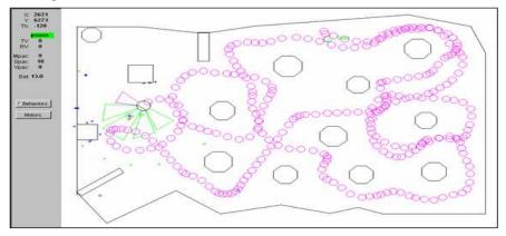
Fig. 31. Trajectories of the robot after the learning of the FIS by algorithm DFQLGA (the third stage)
