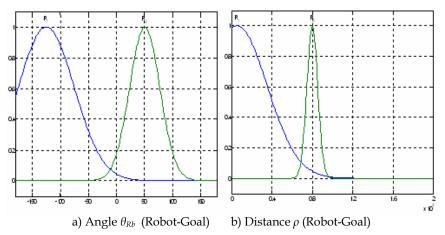
Fig. 20. Determined membership functions after the generation of four fuzzy rules
