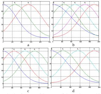
Fig. 26. Final membership functions of the inputs of the FIS determined by the DFQLGAalgorithma) Right Distance,<br/>c) Frontal-Left Distanceb) Right-Frontal Distancec) Frontal-Left Distanced) Left Distance.
