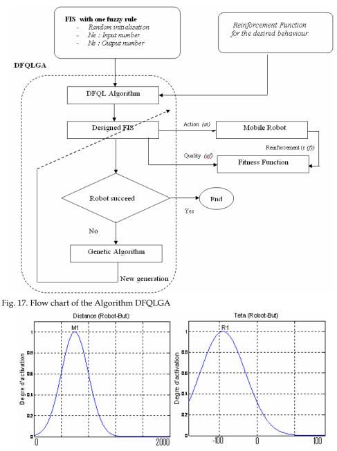
Fig. 18. the initialized membership functions for the two input of the FIS
