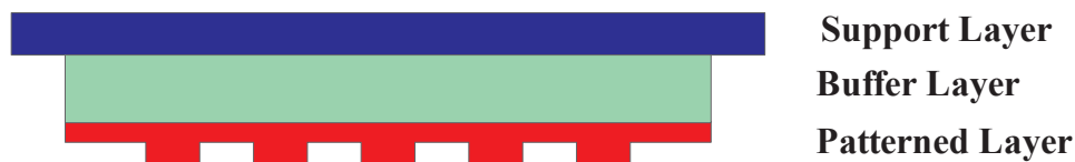
Figure 6. Structural model of a common soft mold
