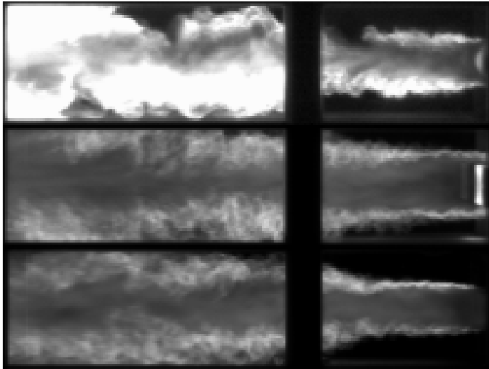
Figure 2. High speed images of the circular cylinder (top), square cylinder (middle) and V gutter (bottom) at Re = 30,000 and stoichiometric mixture [2].
