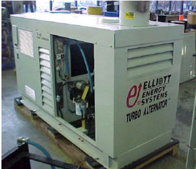
Figure 1. Elliott Energy Systems Microturbine, TA-45 model.
