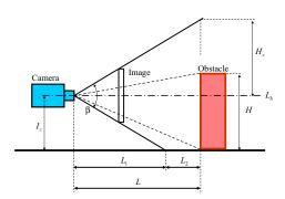
Figure 3. Camera model in side view
