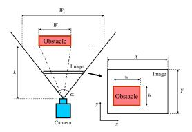
Figure 2. Camera model in top view
