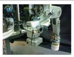
(b) The USB camera fixed to the body of the robot
