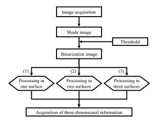
Figure 5. Flow of image data processing
