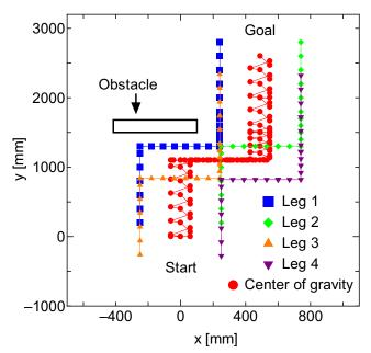
Figure 14. Experimental result of detour action
