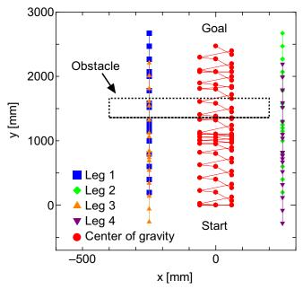
Figure 12. Experimental result of climbing-over action
