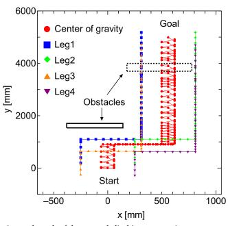
Figure 17. Experimental result of detour and climbing-over action
