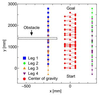
Figure 10. Experimental result of striding action
