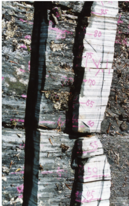
Figure 3. A field photograph of the Dwyer Lake BIF. The light and dark bands on the tabular samples correspond to the Si-rich and Fe-rich mesobands, respectively. The numbers on the sample’s surface denote the distance described in intervals of 5 cm.
