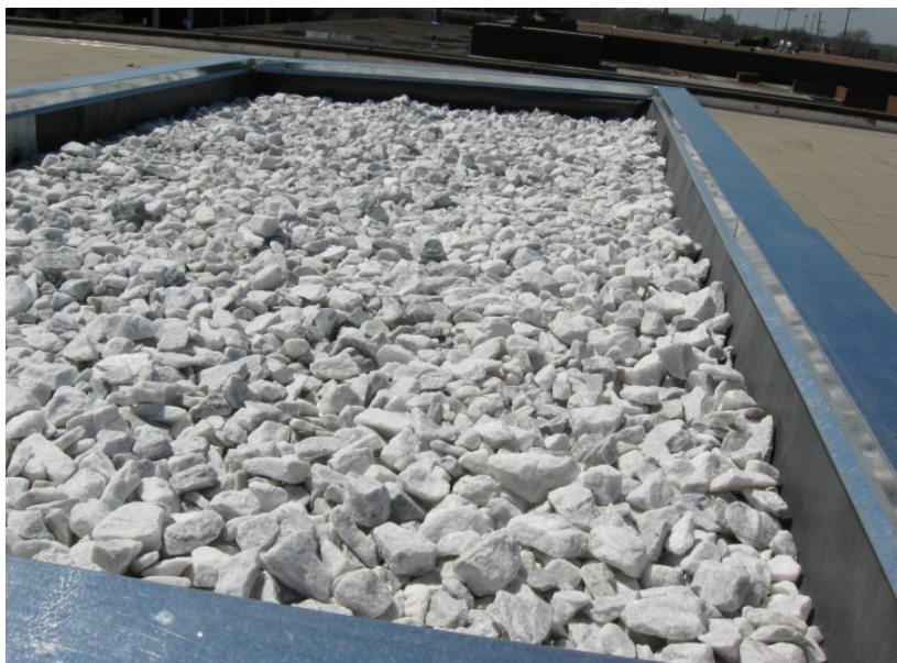
Figure 8. Mini-roof equipped with crushed marble chips.
