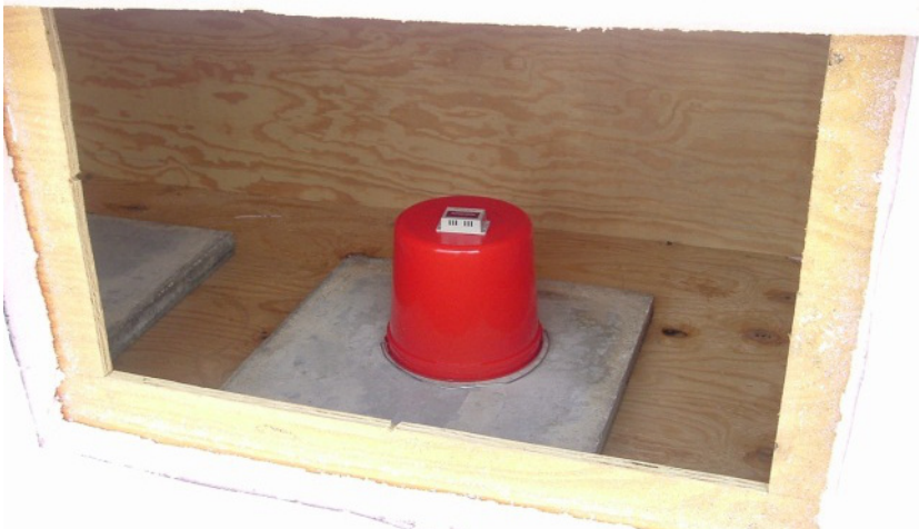
Figure 3. Mini-roof system showing temperature sensor installed inside a mini-roof.
