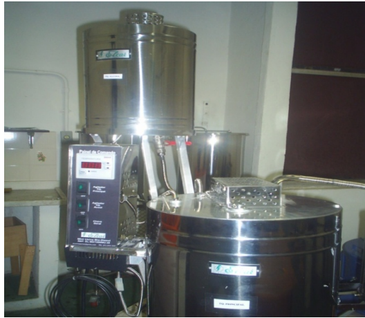
Figure 9. Small plant for the production of biodiesel
