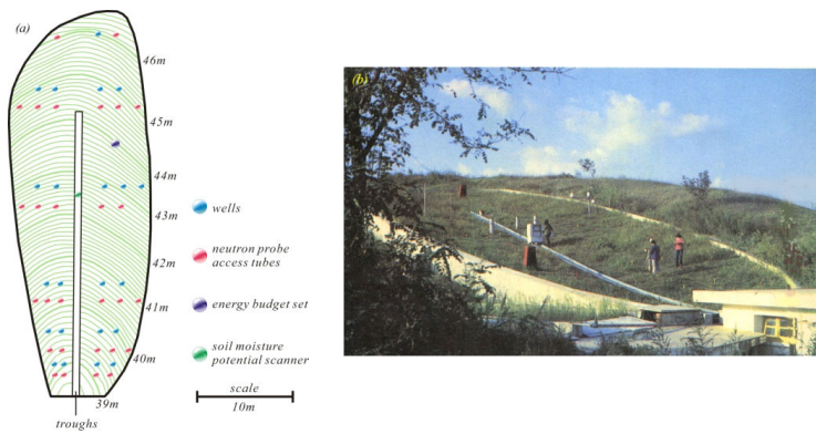
Figure 12. Hydrometric monitoring of Hydrohill. (a) Plan view of the surface topograph showing the locations of groundwater wells, access tubes for neutron moisture probe with potential scanner, the central stacked lysimeter troughs, the energy budget set. (b) Whole view of its surface watershed in operation during early years (1980's), under renovation now.
