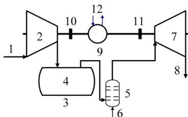
1.Air, 2.Compressor, 3.Reservoir, 4.Compressed air,
