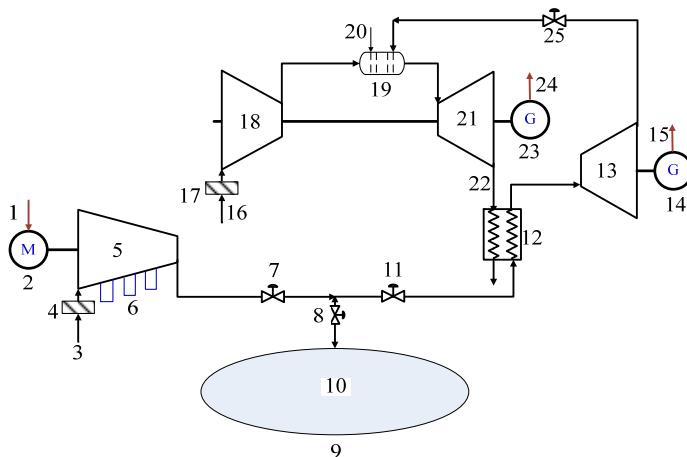
1 15 and 24.Electricity, 2.Motor, 3 and 16.Air, 4 and 17.FltEr, 5 and 18.Compressor, 6.Intercooler, 7 8 11 And 25.Valve, 9.Underground Cavern, 10.Compressed Air, 12.Recuperator, 13 and 21 Turbine, 14 and 23 Generator, 19.Combustor, 20.Fuel, 22.Exhaust
