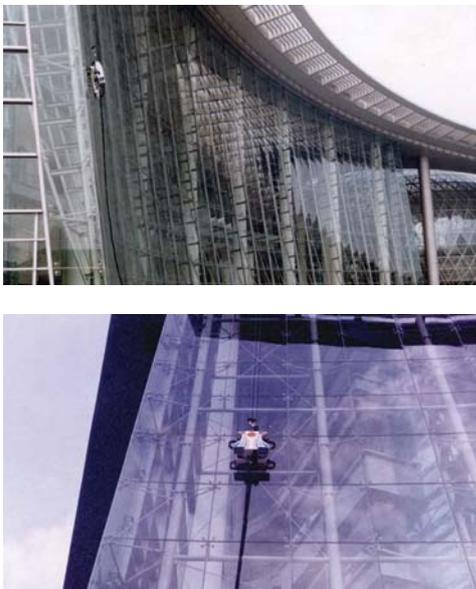
Fig. 16. Sky Cleaner 3 cleaning on the target glass wall
