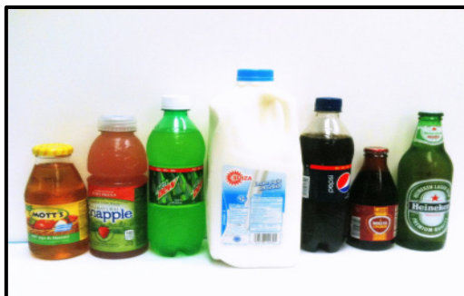
Figure 1. Commercial bottles (glass and plastic) used to TEP detection using Optical Fiber Coupled Raman spectroscopy.
