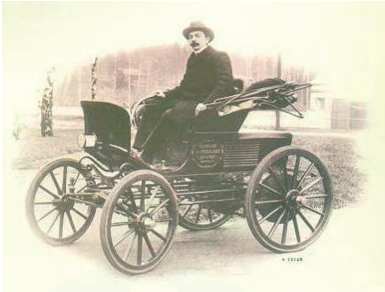
Figure 2. First EV's were possible to cross up to 100 km, moving with speed below 20 km/h.
