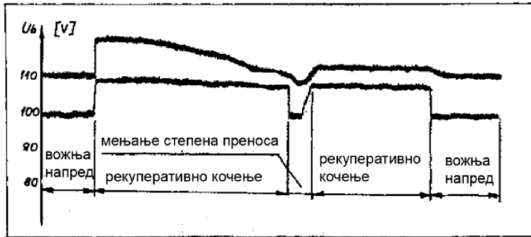
Figure 8. Change the battery voltage during DC recuperative braking in [22, 23].
