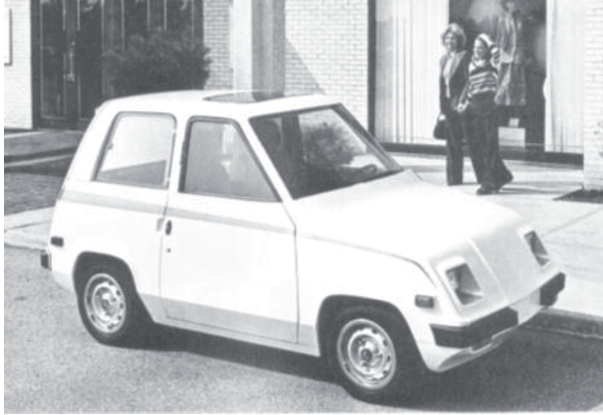
Figure 7. Copper City electric Car Runabout power 15kW made on the basis of cooperation for the use components of Renault R5.
