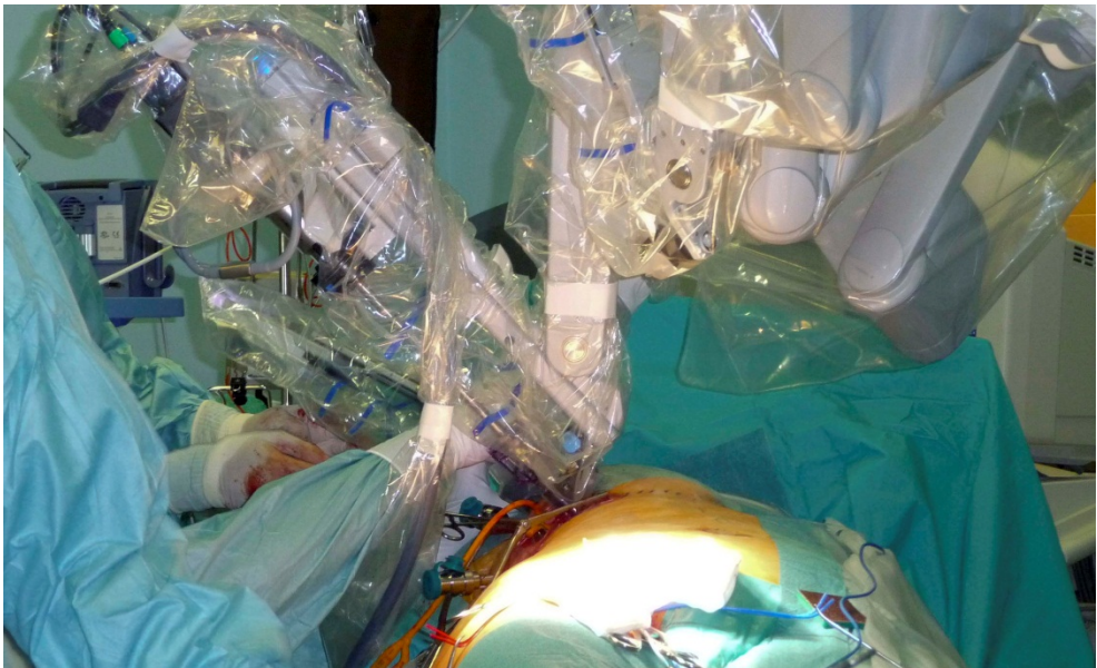
Figure 5. View of the da Vinci robotic system's arms positioned in the patient's chest, for robotic assistance when a thoracotomy incision has been made.
