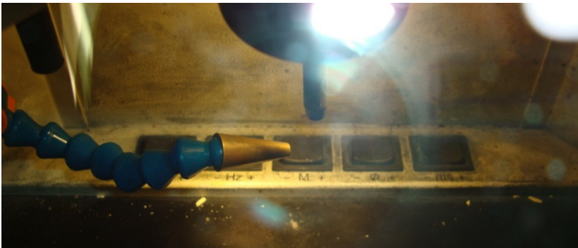
Figure 7. Laser welding machine (output of the light beam and the shielding gas).
