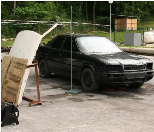
**Figure 1.** Automobile with thermocouples prepared for the experiment
