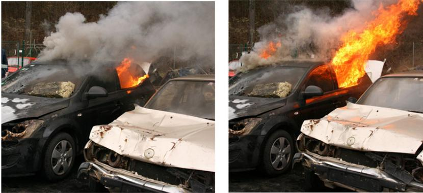
**Figure 12.** Full-scale fire experiment: passenger compartment fire
