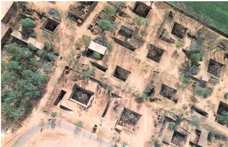
Figure 2. Aerial view of an earth shelter neighborhood in Lian Jiazhuang , Shanxi Province, North-western China
