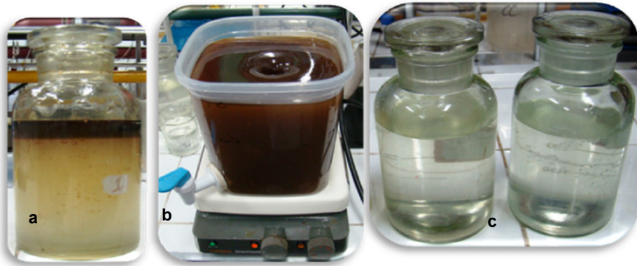
Figure 8. EF tests with high-salinity effluent. Legend: 60g / L NaCl: a) raw wastewater containing 60g / L of O&G; b) raw wastewater being mixed salt, for EF testing; c) effluent treated with AC (left) and DC (right) electroflocculation.
