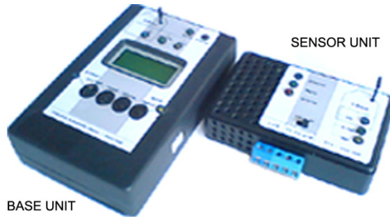
Figure 1. Wireless filter monitoring system
