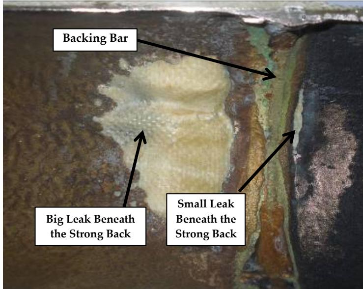
**Figure 2.** Big and small leak near the backing bar at about 6 o'clock position viewed from the inner side of seawater inlet pipe.
