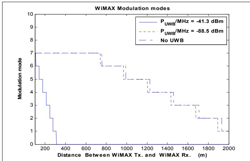
**Figure 3.** 3.5 GHz WiMAX modulation modes for different UWB power densities with a 1 m distance between the UWB transmitter and the WiMAX receiver assuming a WiMAX transmitted power of 40 dBm/sector and that the WiMAX signal and interference are received through an open window.
