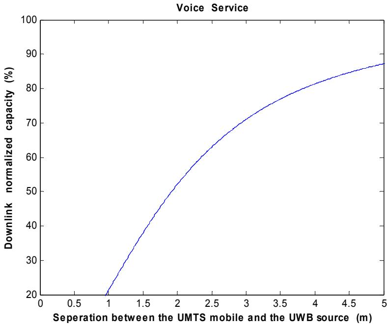
**Figure 11.** Effect of the UWB interference on the macrocell normalized capacity as a function of the separation between the UWB transmitter and the UMTS mobile ( $P_{UWB} = -60 \text{ dBm}/\text{MHz}$ ).
