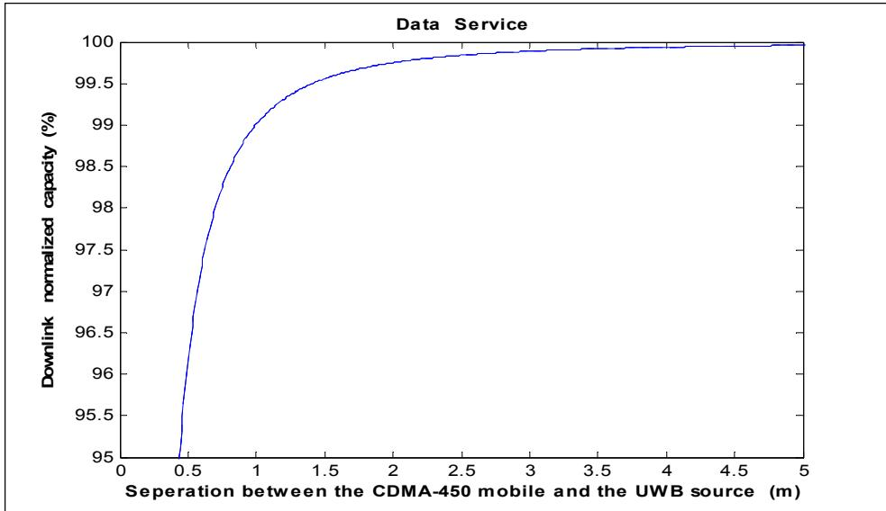
**Figure 17.** Effect of the UWB interference on the macrocell normalized capacity as a function of the separation between the UWB transmitter and the CDMA450 mobile ( $P_{UWB} = -95 \text{ dBm/MHz}$ ).
