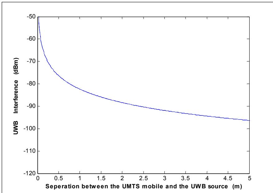
**Figure 9.** UWB interference as a function of the separation between the UWB transmitter and the UMTS mobile ( $P_{\text{UWB}} = -51.3 \text{ dBm/MHz}$ ).
