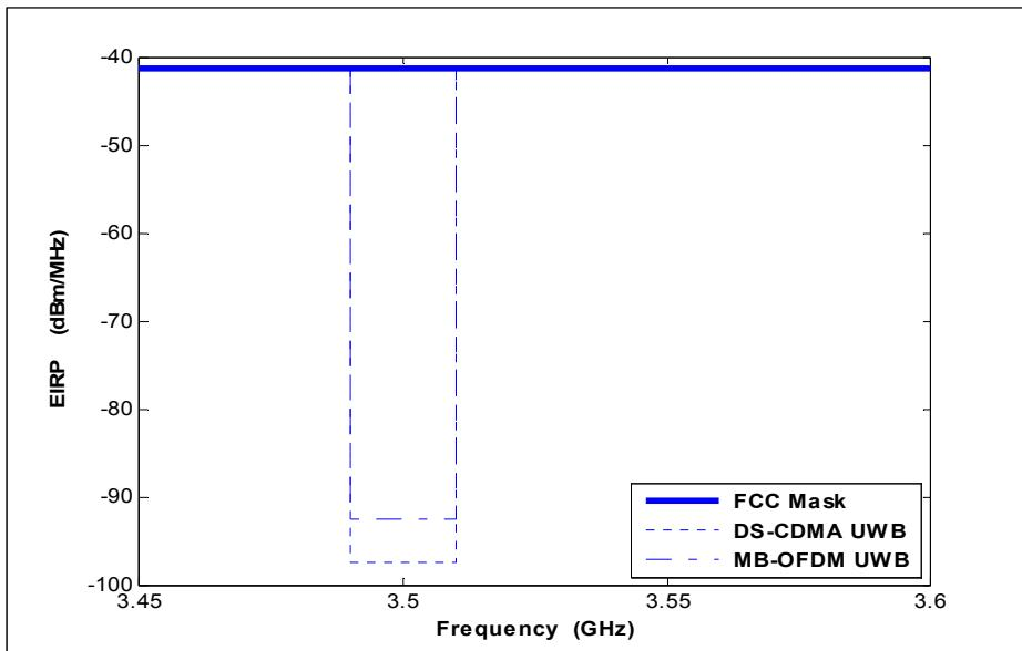
**Figure 8.** DAA requirements within the 3.5 GHz band.
