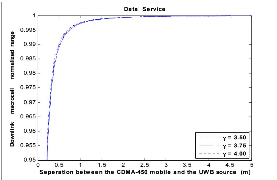
**Figure 16.** Effect of the UWB interference on the macrocell normalized range as a function of the separation between the UWB transmitter and the CDMA450 mobile ( $P_{UWB} = -95 \text{ dBm/MHz}$ ).
