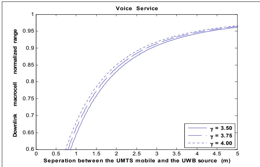
**Figure 10.** Effect of the UWB interference on the macrocell range as a function of the separation between the UWB transmitter and the UMTS mobile ( $P_{UWB} = -51.3\text{dBm}/\text{MHz}$ ).
