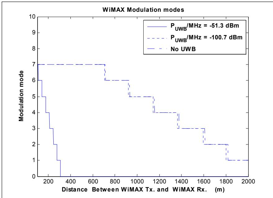
**Figure 7.** 2.5 GHz WiMAX modulation modes for different UWB power densities with a 1 m distance between the 4 UWB transmitters and the WiMAX receiver assuming a WiMAX transmitted power of 40 dBm/sector.
