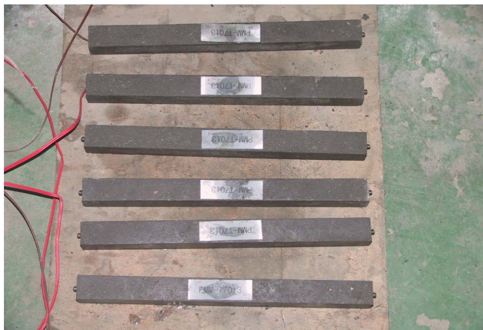
Figure 4. Strain gage setup for length change
