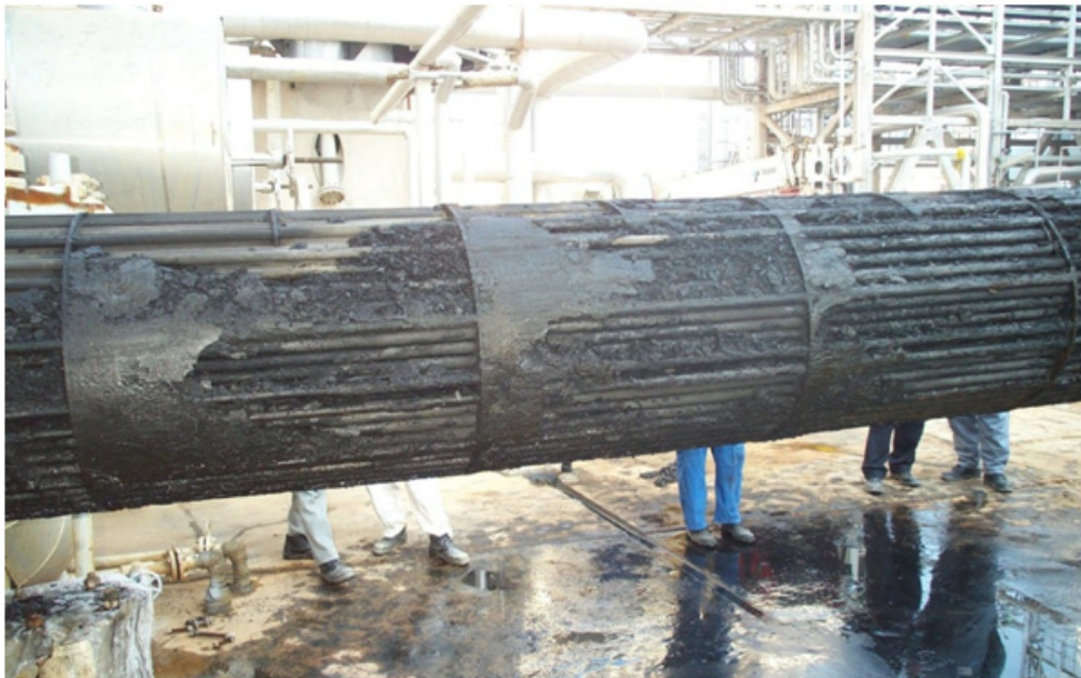
Figure 1. Fouling of heat exchangers.
